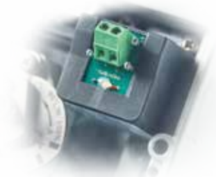
Internal I/p with simple loop test points
